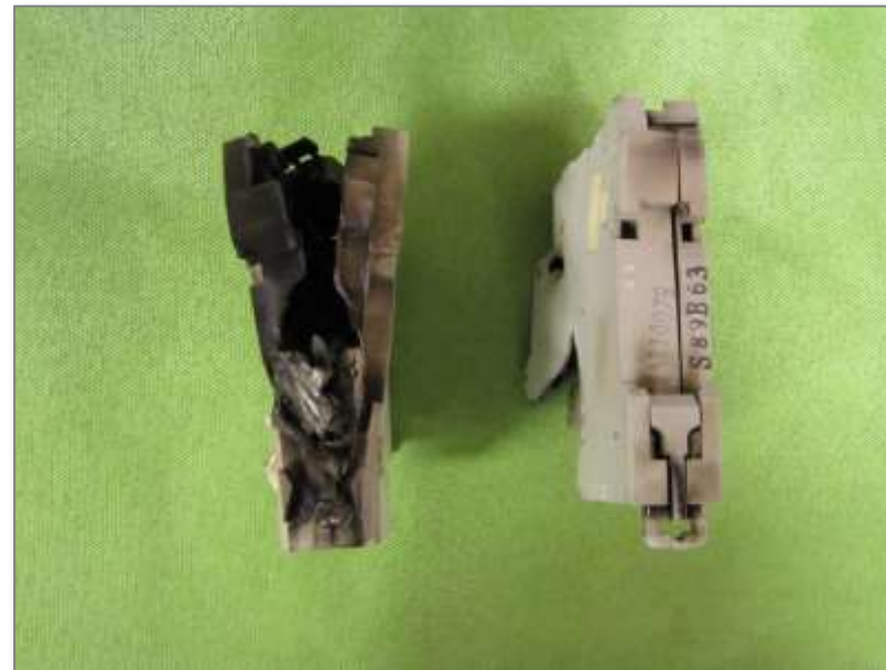
2 Suspect brands of MCB literally 'explode' on Short Circuit test
