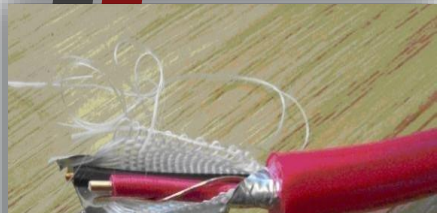
Non-compliant armoured cables
